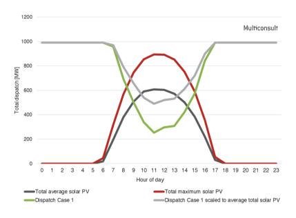
The simulated solar PV profiles and dispatch at the load-following power plant. Dispatch Case 1 is based on the total maximum solar PV profile, while the scaled Dispatch Case 1 is adjusted by the ratio between average and maximum solar profiles. This is to simulate a more moderate case and typical day (based on average) rather than the extreme case.
